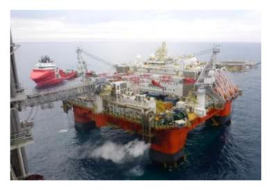
Safe Boreas was built at Jurong Shipyard in Singapore to the GVA 3000E design utilising GVA's extensive semisubmersible design experience. The vessel is designed for worldwide operations in the harshest offshore environments including the North Sea, and can operate both in DP and anchored mode, providing maximum cost efficiency and flexibility.
