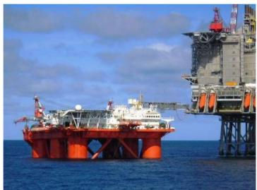
Safe Caledonia is a thruster assisted moored semi-submersible accommodation vessel capable of operating in the most demanding geographical areas and has a UK Safety Case.
