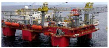
Safe Concordia is a self-propelled semi-submersible accommodation and service vessel of twin hull configuration, capable of operating in benign to moderately harsh environments.
