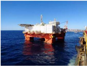
Safe Eurus is a technologically advanced and flexible DP3 semi-submersible ASV designed for worldwide operations, excluding Norway.
