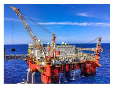
Safe Notos was built at Cosco to an enhanced Gusto MSC's Ocean 500 design incorporating DP3 station keeping systems, 10-point chain mooring and variable draft operations in the harshest offshore environments, excluding Norway.
