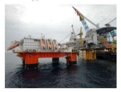
Safe Zephyrus was built at Jurong Shipyard in Singapore to the GVA 3000E design utilising GVA's extensive semi-submersible design experience. The vessel is designed for worldwide operations in the harshest offshore environments, including the North Sea.
