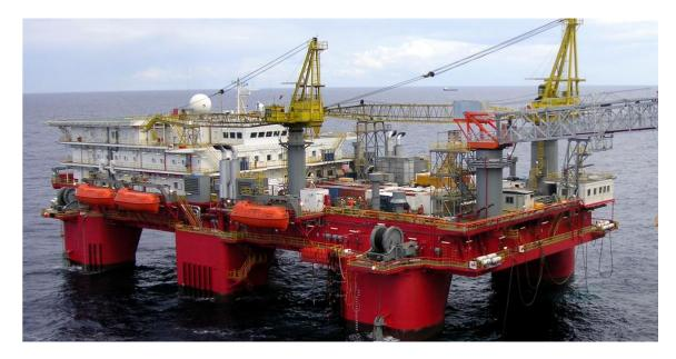
2005 built DP 2 vessel. No substantial life-extension project executed to date
