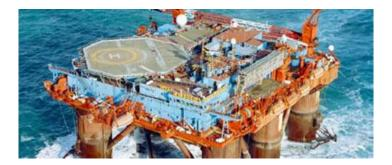
Safe Caledonia is a thruster assisted moored semi-submersible accommodation vessel capable of operating in the most demanding geographical areas.
