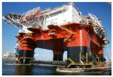
Safe Zephyrus was built at Jurong Shipyard in Singapore to the GVA 3000E design utilising GVA's extensive semi-submersible design experience. The vessel is designed for worldwide operations in the harshest offshore environments, including the North Sea.
