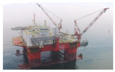
Safe Eurus is a technologically advanced and flexible DP3 semi-submersible ASV designed for worldwide operations, excluding Norway.
