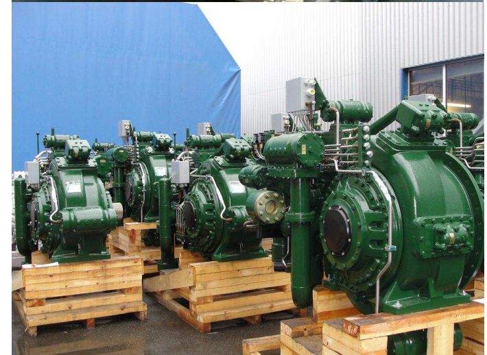
New fairleads and winch motors
